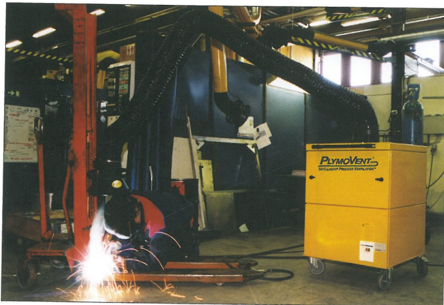
The PlymoVent Extraction arm can be rotated through 360° – reach everywhere!
