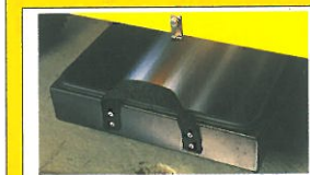
Integrated seal-tite dust tray prevents dust from re-entering or escaping from the filter.
