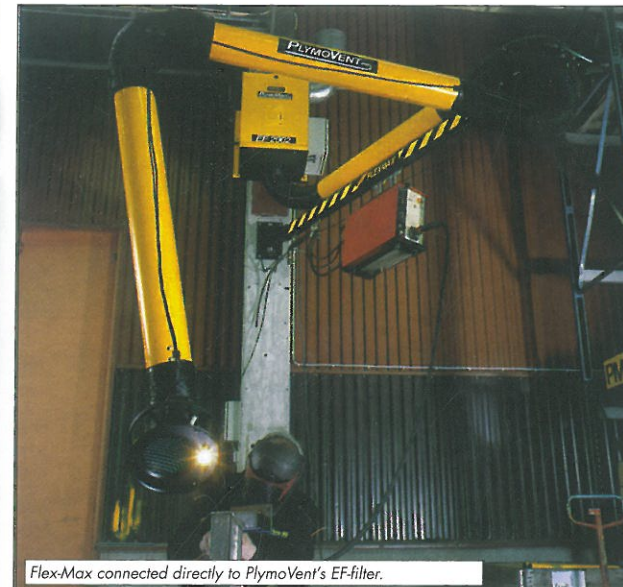
Flex-Max connected directly to PlymoVent's EF-filter.
