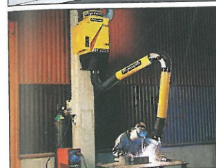
PlymoVent KUA arm mounted directly to an EF filter.
