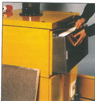
Front access makes the welding filter easy to remove.
