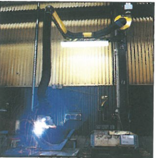
50 kg/110 lbs can be suspended from the inner arm which has a sliding services rail. 10 kg/22 lbs can be suspended from the outer arm. Perfect for tools etc.
